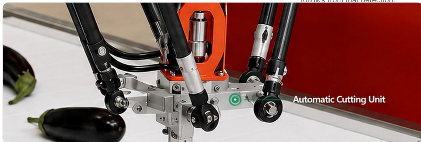
VISION AND CUTTING REGION ABOVE THE PRODUCT CONVEYOR
